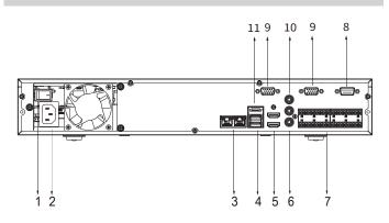
1 Power Switch Power Input 3 Network Ports USB Ports 5 HDMI Ports 6 AUDIO IN, RCA Connector RS-232 Port 7 Alarm In/Out 10 AUDIO OUT, RCA Connector 9 VGA Ports
