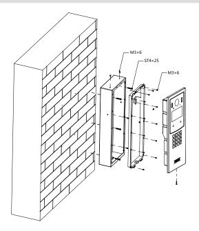
**Step1** Drill holes in the wall according to holes on the surface mount box, and then put expansion tube in the holes.
